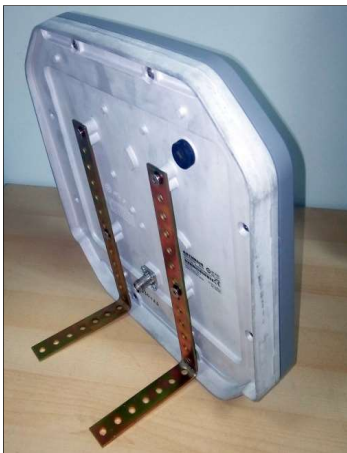
Particular of the metal clamps fixed to antenna. They provide a good stability preserving the correct orientation of the antenna.
